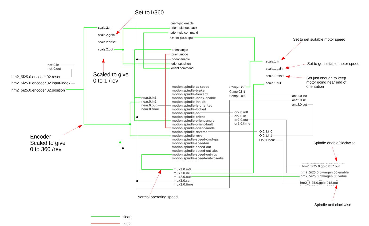
This set up will not work properly with Old Jaguar Cub inverter, as it will not go slow enough for spindle to stop near correct position. A newer drive may be ok. If the speed is set using the inverters own pot, the spindle will stop within two or three degrees. This would be fine for a 24/24 hole 'brake' disc/solenoid to lock spindle.
