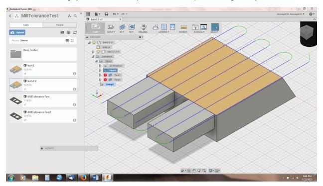
Here is a screenshot of a 3d adaptive toolpath for doing the rest of the machining possible in this orientation.
