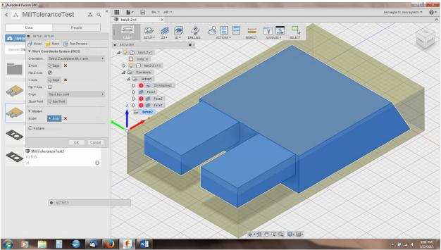
Here is the adaptive toolpath after selecting a tool and keeping other settings as they were.
