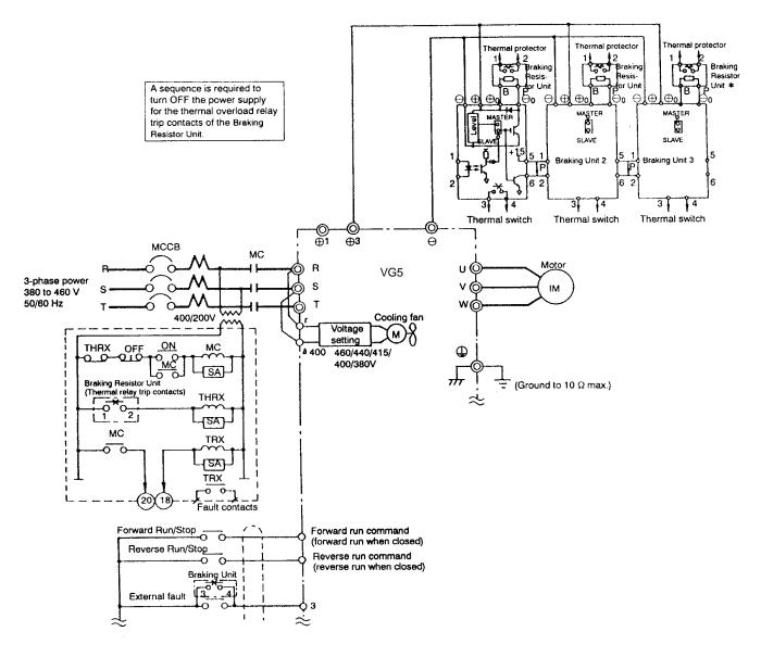
\* Disable stall prevention during deceleration by setting L3-04 to "0" when using a Braking Resistor Unit. The motor may not stop within the deceleration time if this setting is not changed.
