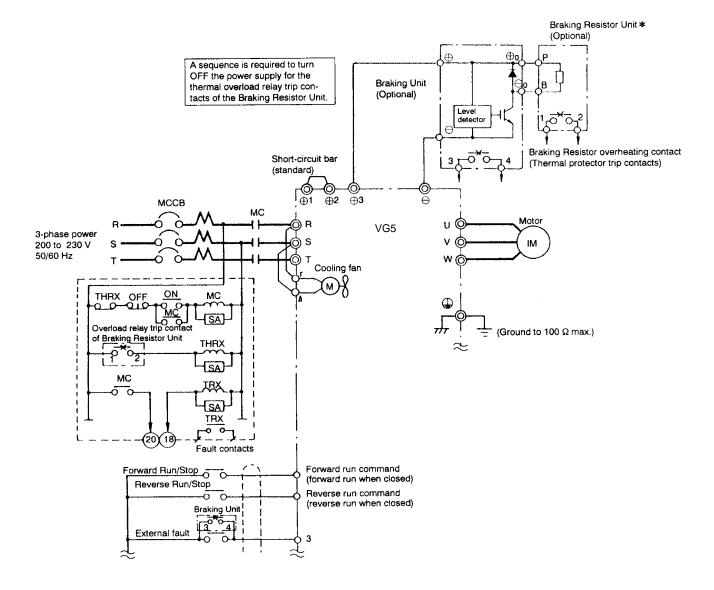
\* Disable stall prevention during deceleration by setting L3-04 to "0" when using a Braking Resistor Unit. The motor may not stop within the deceleration time if this setting is not changed.
