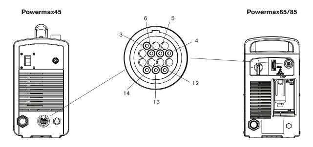
Refer to the following table when connecting the Powermax system to a torch height controller or CNC controller with a machine interface cable.
