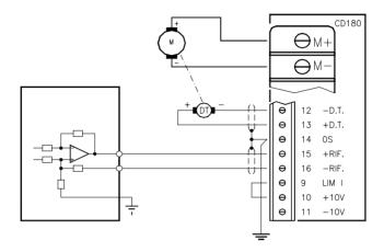
Example with speed control in common mode output stadio.
