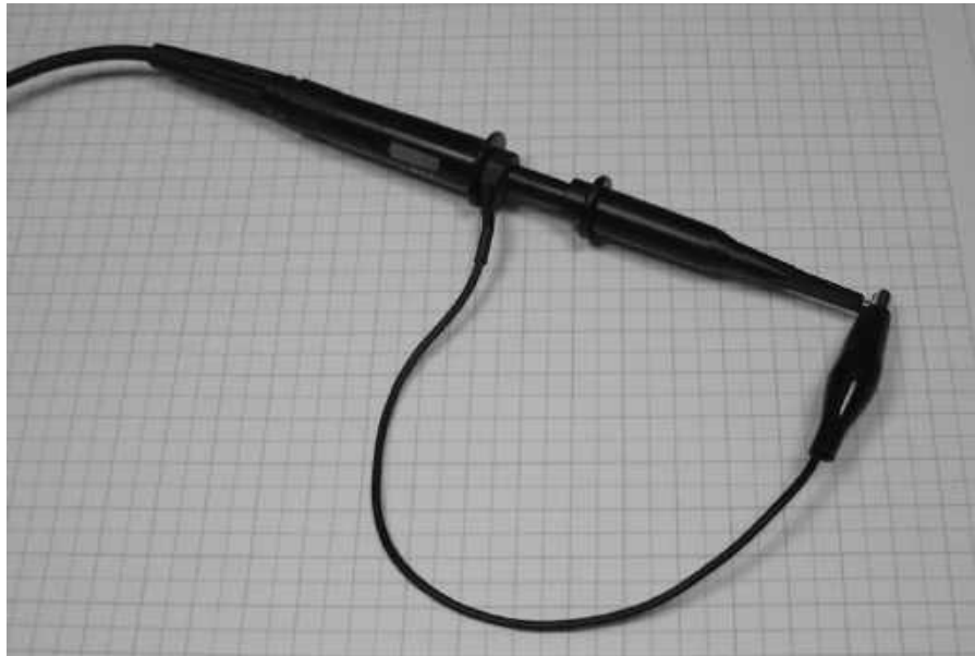
Figure 11.2 Simple H-field probe
