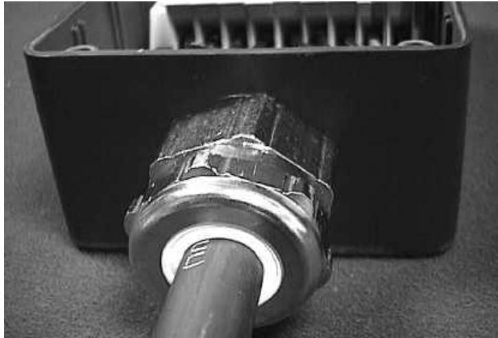
Figure A.3 Gland clamping method
