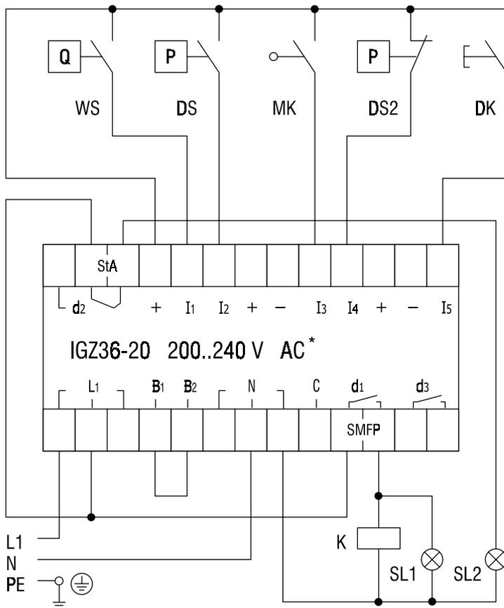
**Figure 2 - 4. Connection Diagram for IGZ36-20**
