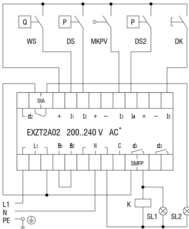
**Figure 2 - 1. Connection Diagram for EXZT2A02**
