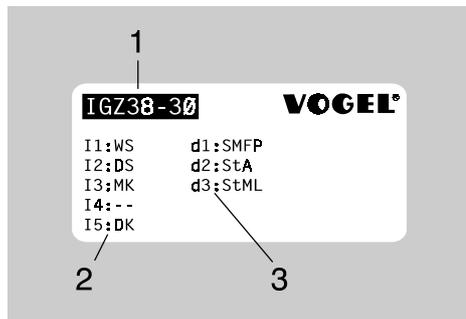
**Figure 1 - 4. Sticker with Information about the Input and Output Assignments**
