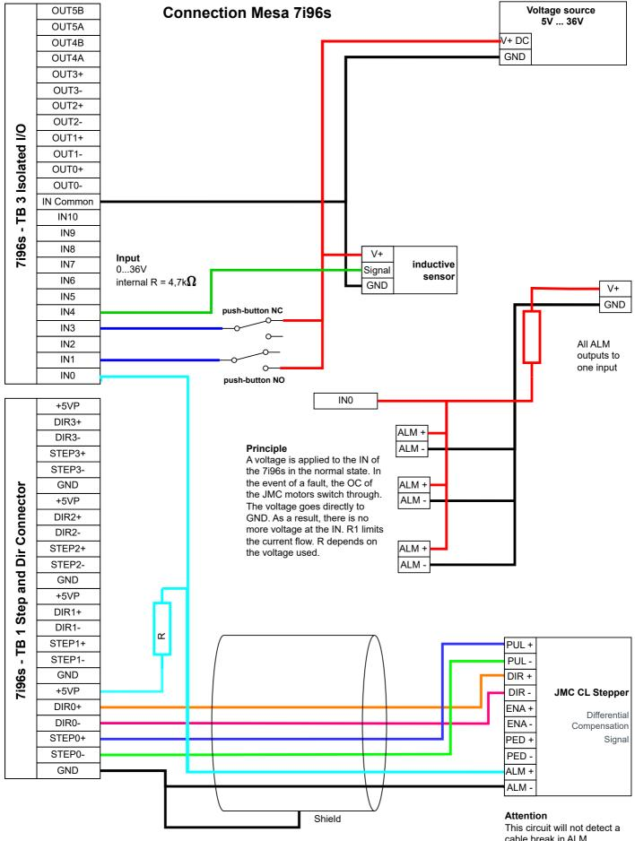
This circuit will not detect a cable break in ALM. However, a cable break in Step / Dir is also not detected.
