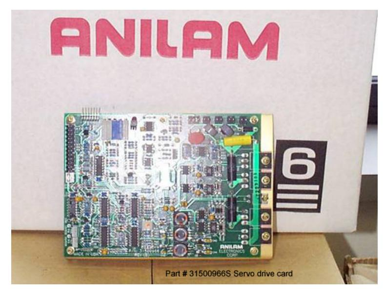
On the top left hand side referenced to the photo, there are 7 test pins. Pin 1 is on the far left this is the common pin. All measurements are referenced to pin 1!
