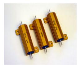
Hi Torque at Top Speed is achieved by over-voltaging the motors with current-limiting power resistors to keep current at the desired level. The resistors do get hot and must be mounted to a heat sink. (Heat sink is not included, a simple sheet of metal will do.) These aluminum frame resistors include mounting holes.
