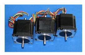
Three NEW NEMA 23 motors, with 1/4" dual-shaft. Motors run smoothly without resonance in the full operational range. Rated 110 oz. in. Top speed is approx 48,000 pulses per minute, which equals 250 rpm, no load condition. Torque is excellent all the way up to top speed. Motors can be run from 5v without power resistors, or 12v with power resistors (resistors for 12v operation are included).
