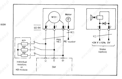
\* short circuit braking for E.Stop condition
