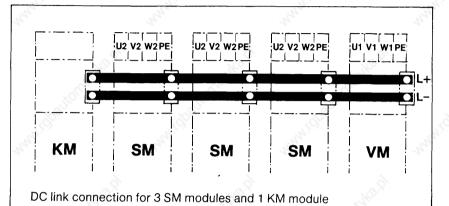
Establish the DC link connection with the busbars and fastening screws supplied in the accessories pack.
