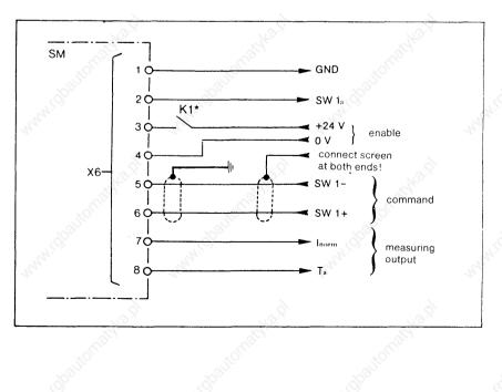
\* Interlocking with K1 (mains and braking contactor) must be provided of that the enable signal is switched off during short circuit braking.
