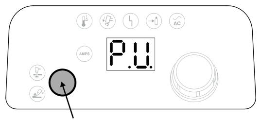
Press-and-hold for 15 seconds to toggle between  ${\bf psi}$  and  ${\bf bar}$ .
